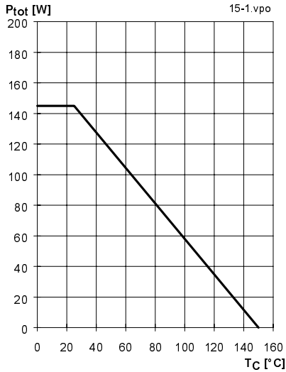
Fig. 1 Rated power dissipation P_{tot} = f(T_C)
